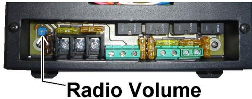
First set the volume level of the vehicle's two-way radio to its normal operating volume. Turn on the On/Off switch of the hand held controller and press the RADIO button. The radio should be rebroadcasting through the siren speaker(s). Using a small flat blade screwdriver, adjust the potentiometer as desired.
